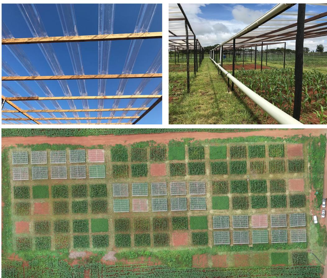
Figure 2. Rainfall exclusion system (top) and aerial view of the University of Zimbabwe Farm (UZF) trial (bottom).
